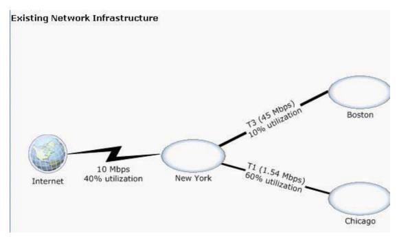
All Internet access is provided through a proxy server located in the New York office. The proxy server provides Internet name resolution on behalf of the client computers.
