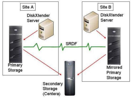
ABC.com is using EMC DiskXtender for Windows at Site A to archive data to an EMC Centera. They are mirroring the primary storage using SRDF. EMC DiskXtender is also installed on Site B to archive the mirrored primary storage. They are archiving the data from both sites to the same virtual pool on the EMC Centera.
