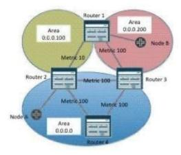
The four routers in the exhibit are participating in a multi-area OSPF topology. Node B (in the upper right-hand corner) is an ASBR advertising an external route. Node A (lower left-hand corner) receives the external route and begins to forward traffic to the ASBR.
