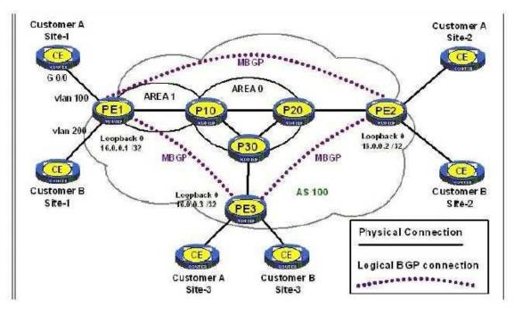
A provider of MPLS services configures MPLS Layer-3 VPN services for two customers. Each customer has three branch offices that will be interconnected by MPLS Layer-3 VPNs. The address blocks chosen by the customers for each site are shown in the following chart: The provider uses OSPF as its IGP with the Loopback 0 addresses shown as the OSPF router-id and the MPLS LSR-ID. A traceroute from Cust-A Site #1 to Cust-A Site #2 displays 5 intermediate routers.
