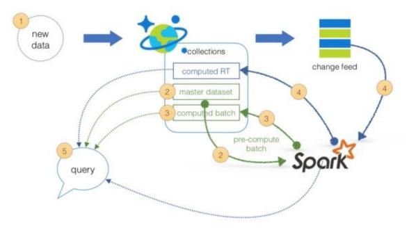
Note: Lambda architecture is a data-processing architecture designed to handle massive quantities of data by taking advantage of both batch processing and stream processing methods, and minimizing the latency involved in querying big data. References:
