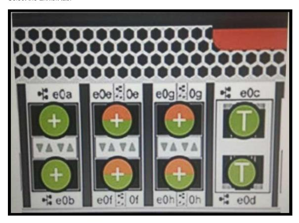
You finished the installation of a new FAS8200 system. The customer wants to use FC and 10G Ethernet but only has the onboard UTA2 ports available. Referring to the exhibit, which two sets of ports would the customer use? (Choose two.)
