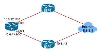
So if we don't specify the source IP, R1 will ping via E0/0 to ISP1. If the ping fails, R1 will remove the first default route so the backup path via ISP2 will be used and traffic will be sent via E0/1. But it also makes the track UP again (as we did not specify the source IP) and the main path is installed again to the routing table -> The connection will flap between two ISPs.
