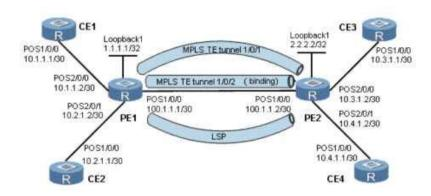
This figure shows the MPLS L3VPN networking. CE 1 and CE 3 belong to VPN A. CE 2 and CE 4 belong to VPN B. Two MPLS TE tunnels (5 Mbit/s and 10 Mbit/s) and an LSP tunnel are set up between PE 1 and PE 2.It is expected that a tunnel policy is configured on PE 1 to distribute traffic in the three tunnels and MPLS TE tunnels are preferred. Configurations on PE1:
