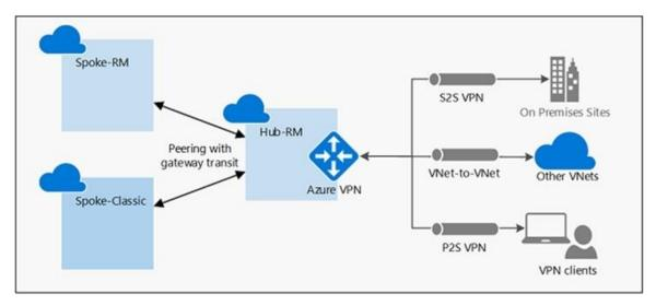
In the diagram, gateway transit allows the peered virtual networks to use the Azure VPN gateway in Hub-RM. Connectivity available on the VPN gateway, including S2S, P2S, and VNet-to-VNet connections,
