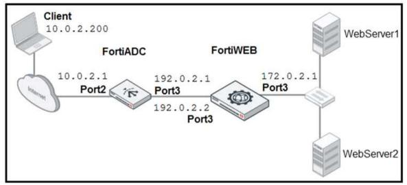
FortiADC is applying SNAT to all inbound traffic going to the servers. When an attack occurs, FortiWeb blocks traffic based on the 192.0.2.1 source IP address, which belongs to FortiADC. The setup is breaking all connectivity and genuine clients are not able to access the servers. What must the administrator do to avoid this problem? (Choose two.)
