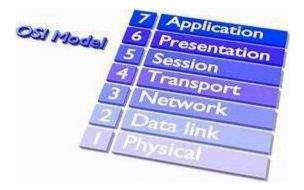
During the data encapsulation process, the Data Link layer of the OSI model is responsible for adding a header that contains MAC addressing information and a trailer used for error checking. The header typically includes the source and destination MAC addresses, while the trailer contains a Frame Check Sequence (FCS) which is used for error detection.
